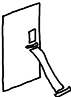
Figure 4.1: Using bracing to secure a door
